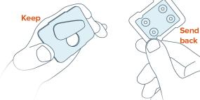
\*WARNING: Piercing, opening, tearing, or cutting the blister pack may cause permanent damage to the internal components of your dosimeter—rendering it unable to accurately and effectively measure dose. Damaged Blister Packs may incur a damage fee.
